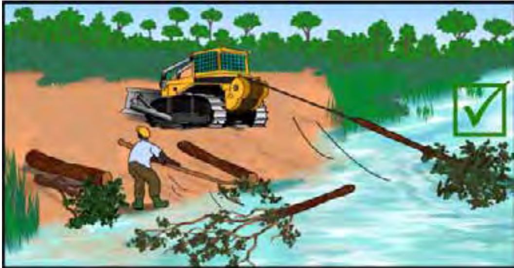
Figure 45: remove tree tops and debris from water bodies
