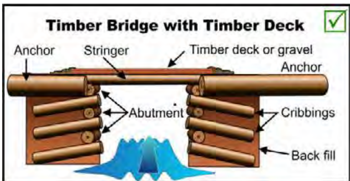
Figure 68: Example of large timber bridge
