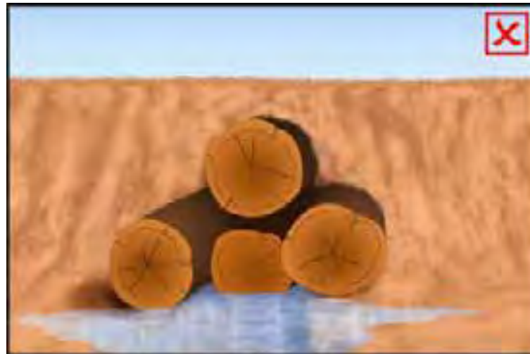
Figure 66: Log clusters with earth fill are not allowed
