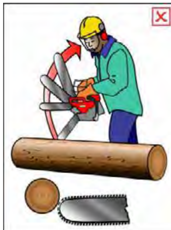
Figure 32: Avoid cutting with the upper tip of the guide bar to prevent kickback
