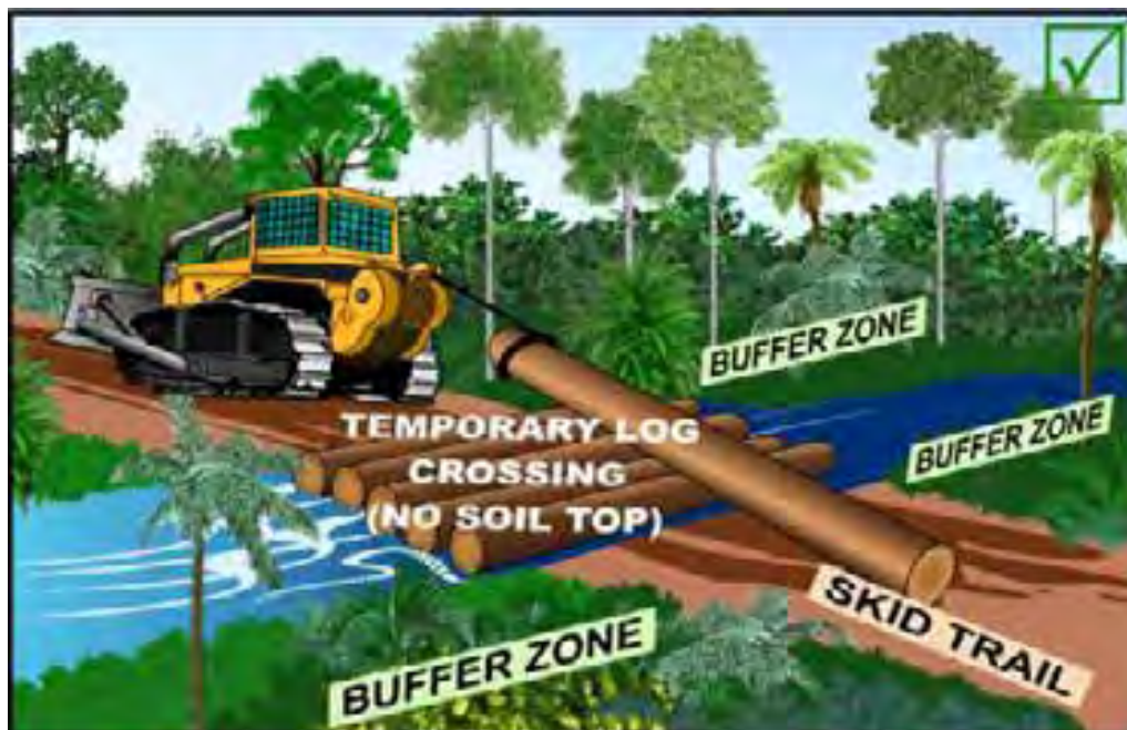
Figure 46: Stream crossing during skidding operations
