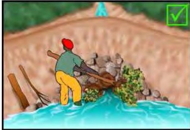
Figure 77: Keep culverts clean during the rainy season
