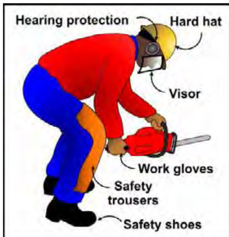
Figure 8: Personal protection equipment required by the operator
