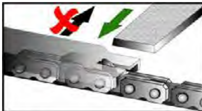
Figure 18: Use flat file to trim off the depth gauge
