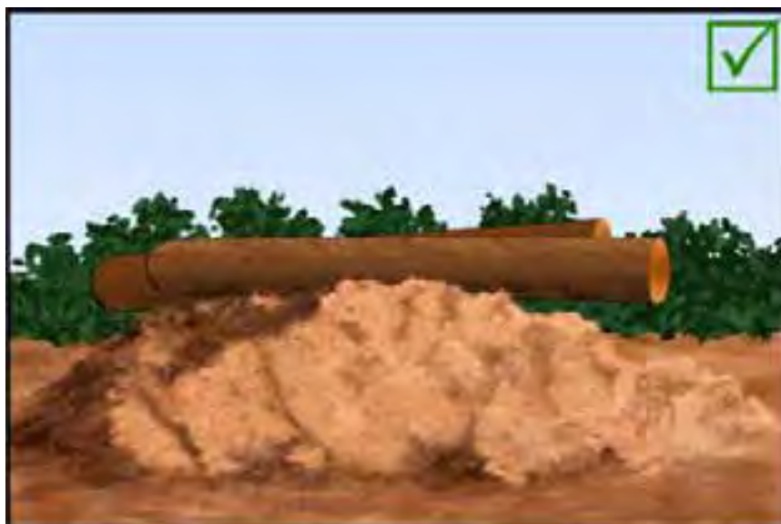
Figure 30: Elevated ramp on landing to facilitate cross cutting
