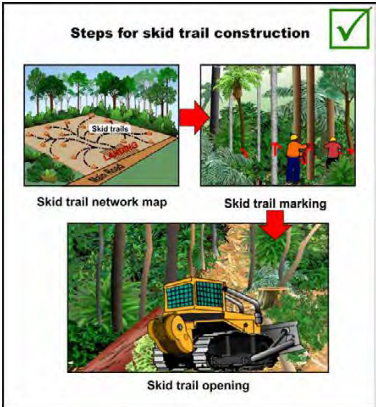
Figure 14: Key steps in preparing skid trails
